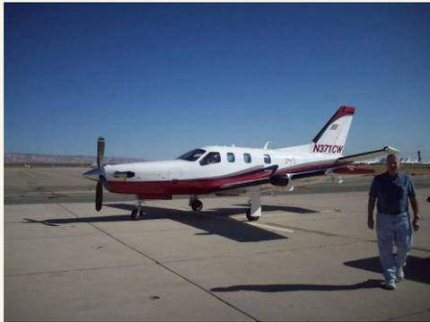
The French made Daher-Socata TBM-850 is the world's fastest single-engine turboprop, with a maximum cruise speed of 320 Knots true airspeed (TAS) at 26,000-feet, with a PT-6 turboprop powerplant.
